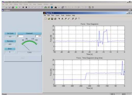
Picture 3: User interface for the the control and visualization of the backstay force measurement. Writer functionality: above: current measured values, below: long-term curvature.
